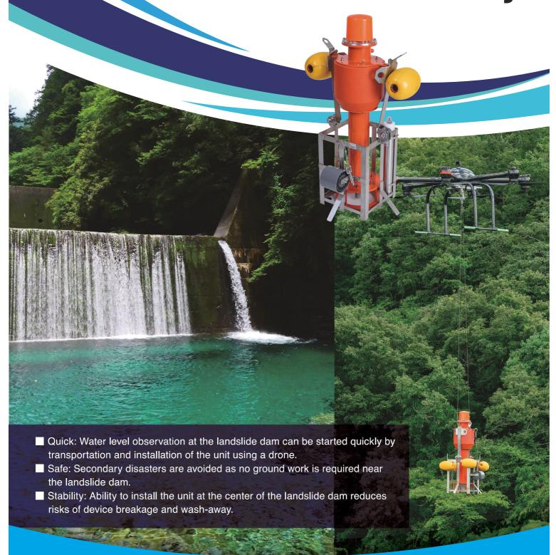
To measure the water level, this device is designed for transportation and installation using a drone when accessing a target landslide dam is difficult due to, for example, disruptions of road caused by a natural disaster.
