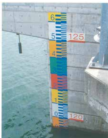
Example: Staff gauge for Dam
