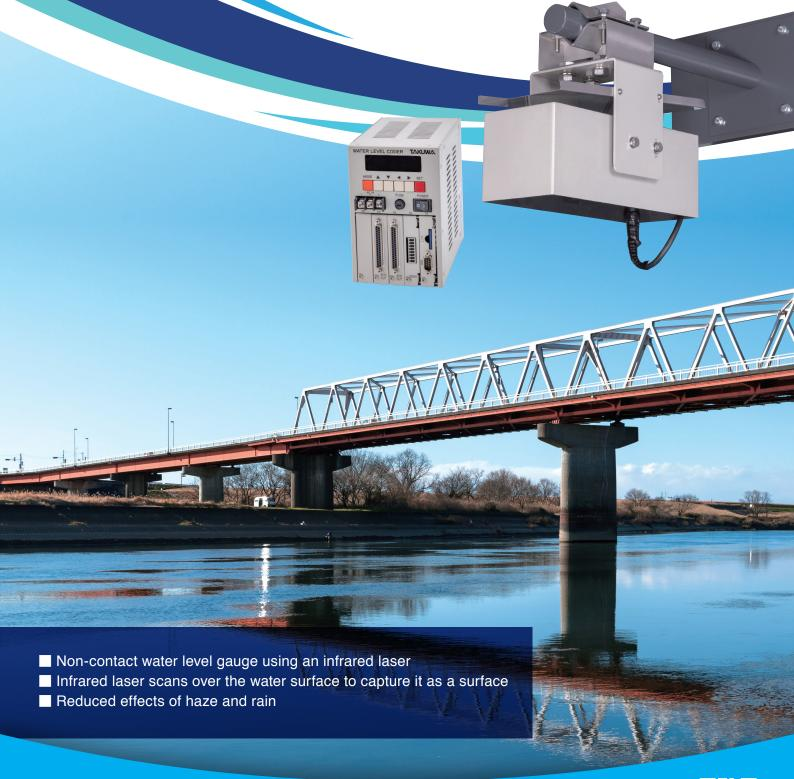
The distance to the water surface is measured based on the infrared laser propagation time from the reflection to the reception of the infrared laser exposed to the surface. The water level is calculated by subtracting this distance from the height of sensor installation position. Compared to our previous models, effects of rain and fog are reduced by scanning the infrared laser over the water surface to capture it as a surface.
